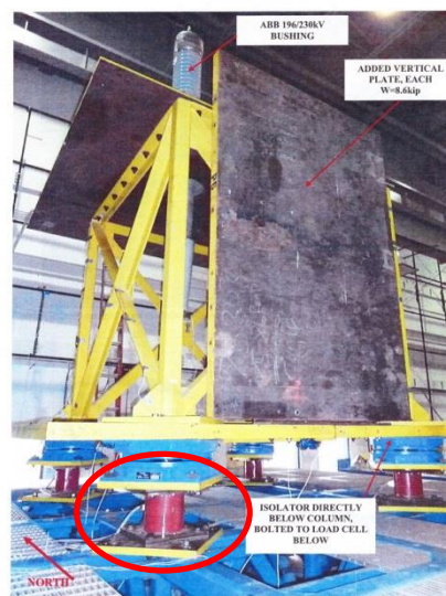
Figure 12 View Model with Full Size Triple Friction Pendulum Bearings on Shake Table
