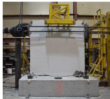
Fig. 2 – Response of Wall SQ1: (a) Force-Displacement Response; and (b) Damage at Ultimate
