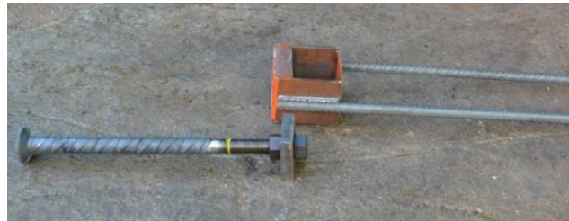
Fig. 12 – Constitutive parts of the wall shoe connection: bolt, washer and nut (bottom left); wall shoe and anchor bars (top right).
