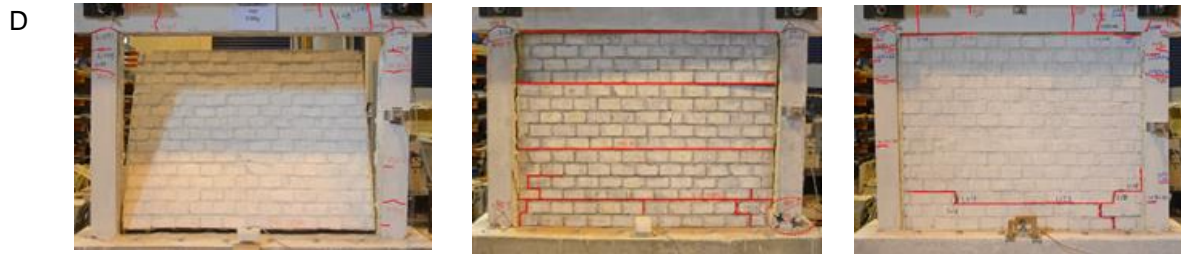
(d). INC, IFC1, IFC2 after 1-g sine wave excitation
