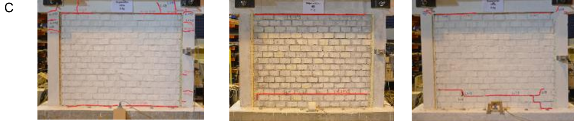
(c). INC, IFC1 and IFC2 after 0.9g, 94% Superstition Hill earthquake, drift ratio 2.71%, 1.73% and 1.88% respectively
