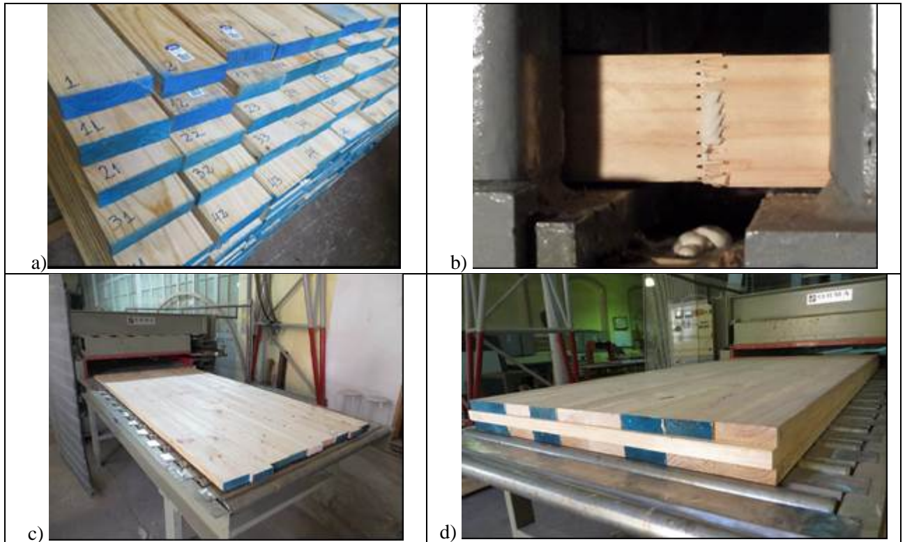
Fig. 3 – Manufacturing process of a radiata pine CLT panel showing a) a sample of sawn lumber used for the panel's layers; b) connections of sawn lumber (typical finger-joint); c) pressing of a layer, and d) final CLT panel.
