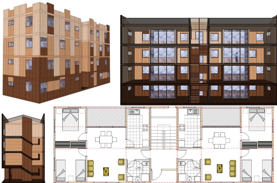
Fig. 6 – Four story building based on CLT projected for social housing in Santiago, showing a) a perspective view; b) a typical elevation; and c) the floor plan of the first story.
