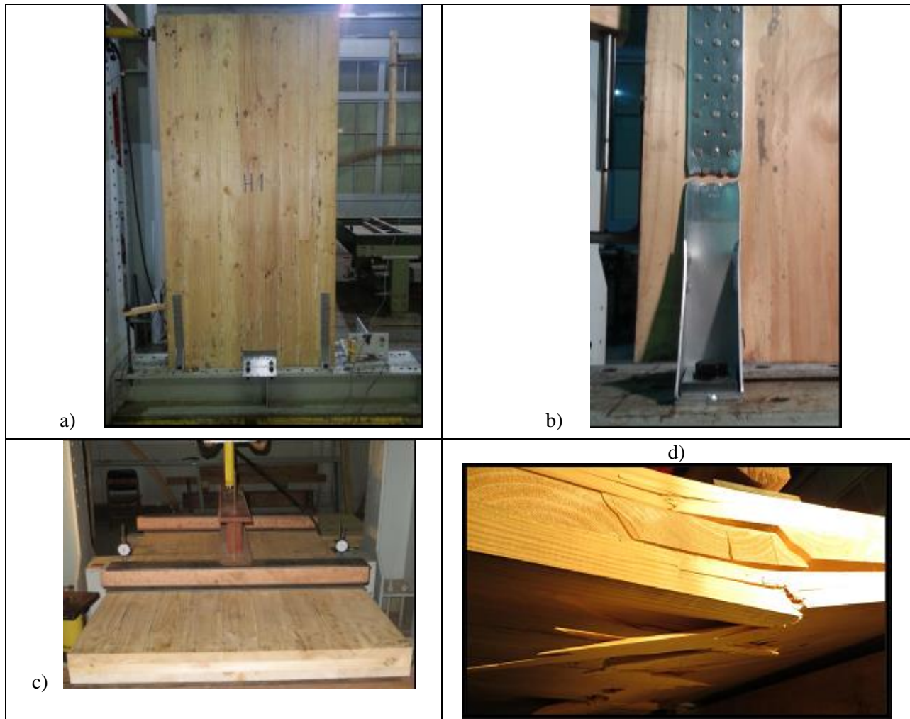
Fig. 4 – CLT panels to be tested under vertical and horizontal loads according to the requirements of Chilean code NCh801 (1971), showing a) the original panel; b) failure of a connection during a test; c) applied load during the bending test; and c) typical out-of-plane failure.
