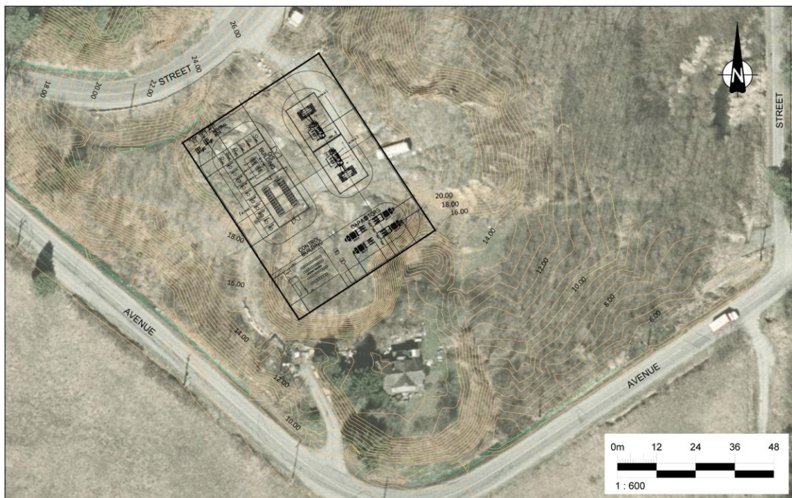
Fig. 1 – Substation Layout Plan
