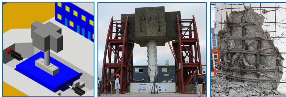
Fig. 1 –Test setup scheme, column after EQ9 and rebar fracture close-up. Photos provided via NEEShub < https://nees.org/warehouse/project/987 >
