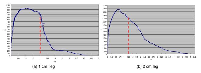
Figure 6. Force-Displacement curve of B&Q on wood.
