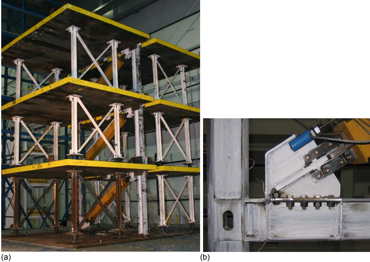
Figure 9. (a) Three-story Shake-Table Test Specimen; (b) removable and eccentric gusset plates (Vargas and Bruneau 2006b).
