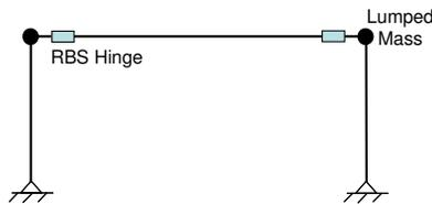
Figure 7. 1D Model with Plastic Hinges.
