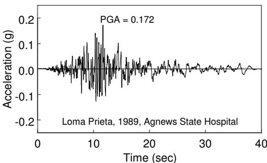
Figure 9. Earthquake record used for analyses.
