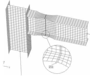
Figure 12. Refined mesh at region most susceptible to low cycle fatigue.
