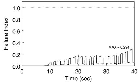
Figure 16. Failure index at RBS connection.
