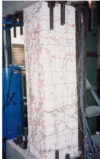
Photo 1. No.4 Specimen loaded at the relative displacement angle R = 1/25
