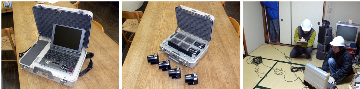
Figure 2 Portable Vibration Measurement Machine, Velocity-meters and view of Microtremor measurement.
