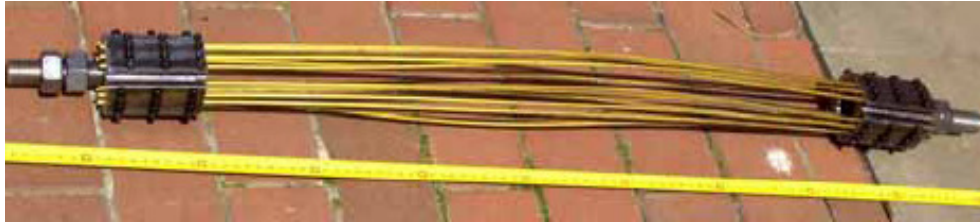
Figure 2. Damper made of several SMA wires developed for family houses (Torra et al. 2006).
