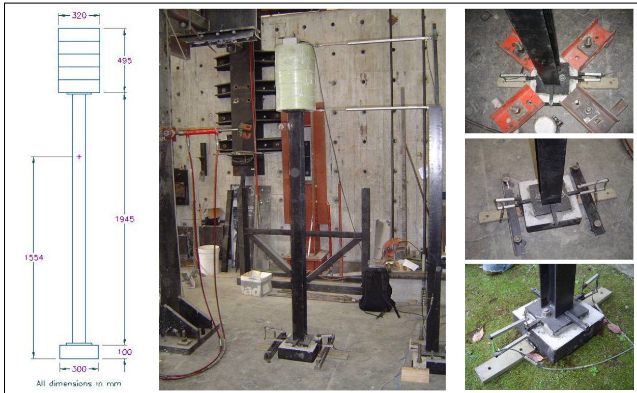
Figure 1. The column test rig used to conduct free vibration/rocking experiments and the three restrain conditions rigid footing, rocking on concrete and rocking on soil.
