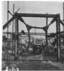
Figure 14. Full scale test of Metallic Damper.
