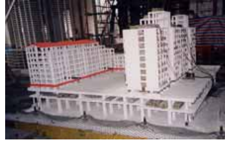
Figure 13. Shaking table tests Isolation structural model.
