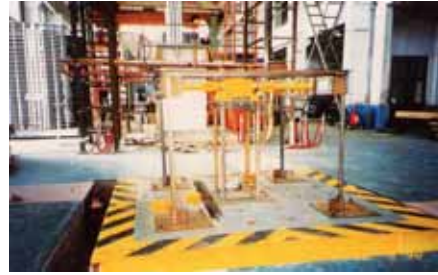
Figure 27. Shaking Table test for AVSD System.
