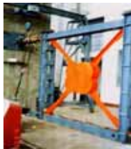
Figure 16. Full scale test of Friction Damper.
