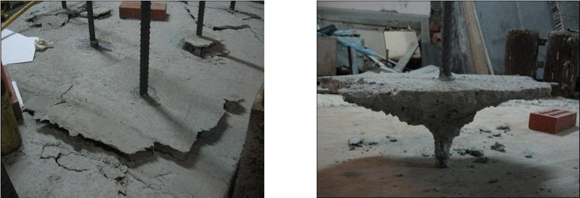
Figure 7. Combined failure mode.
