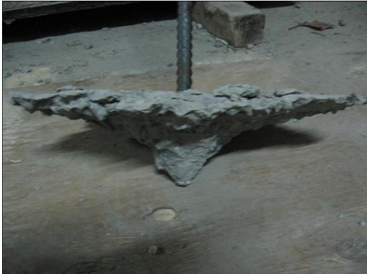
Figure 5. Concrete cone failure in shallow anchors.
