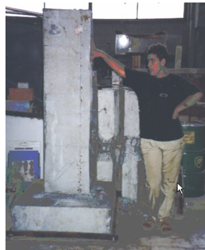
Figure 2b. Bridge pier model specimen tested at the laboratory.
