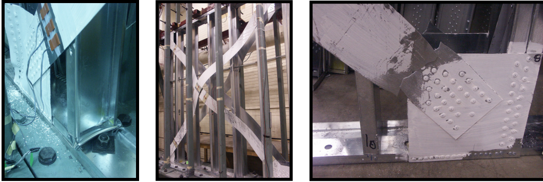
Figure 5. Track compression/bearing, brace yielding and net section fracture failure modes.
