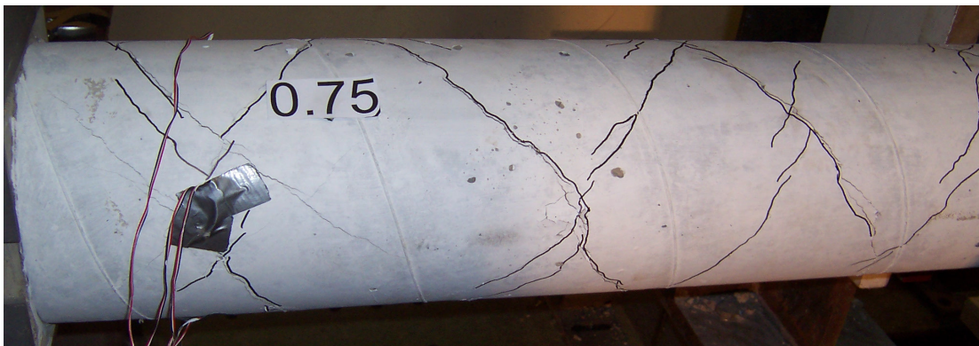
Figure 5. Typical 45° concrete crack angle.
