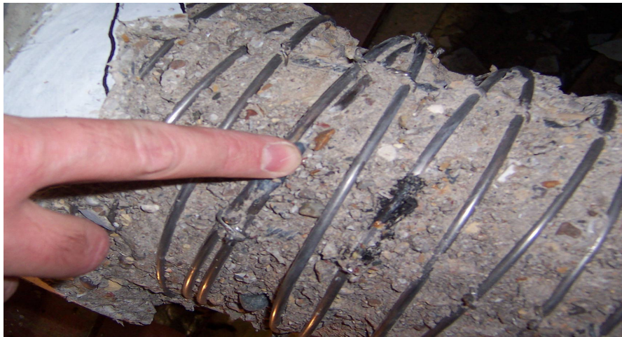
Figure 6. Spiral rupture (35-X).
