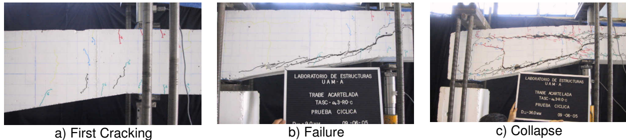
Figure 9. Defined damage states for beams TASC \alpha i-R0-c (illustrated with TASC \alpha 3-R0-c).
