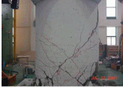
Figure 5. Failure of MS-HT4-N-SH.
