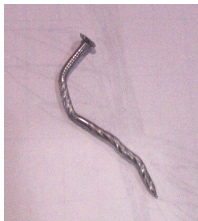
Figure 5. Typical nail failure mode exhibited in walls 704 to 706 with 25.4 mm thick plywood.
