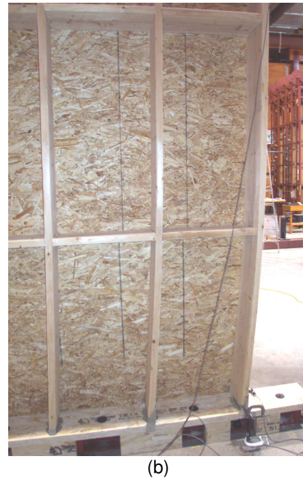
Figure 4. a) Energy dissipation of various walls obtained during the testing; b) Typical deformed shape of the wall studs in the lower half of the walls.
