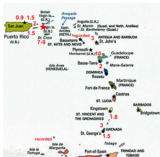
Figure 4. Observed runup amplitudes (m) during the 1867 tsunami, taken from (Zahibo et al, 2003)
