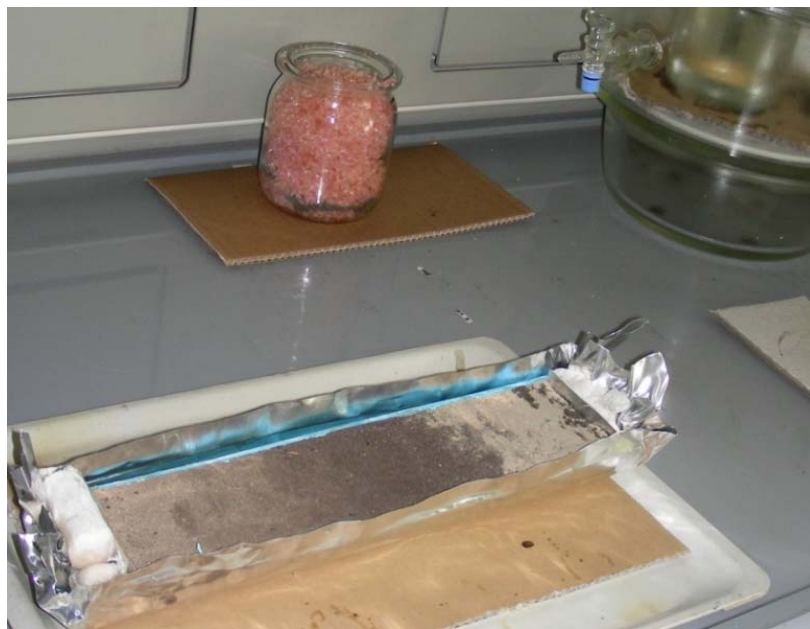
Figure 3. The preparation of core soft sediment for the hardened samples
