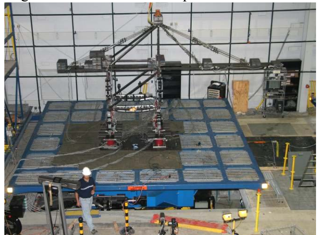
Figure 6. Testing of a 1/20 th scale model of a container crane on one of the NEES shake tables at the University at Buffalo.
