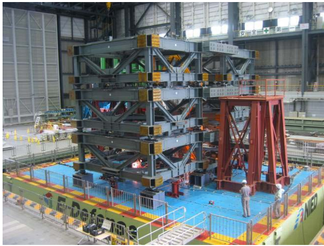
Figure 4. Testing the performance of a damage-tolerant rocking steel frame on the E-Defense shake table near Kobe, Japan.
