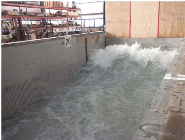
Figure 7. Experimental tsunami bore impacting instrumented wall specimen in NEES Large Wave Flume at Oregon State University.
