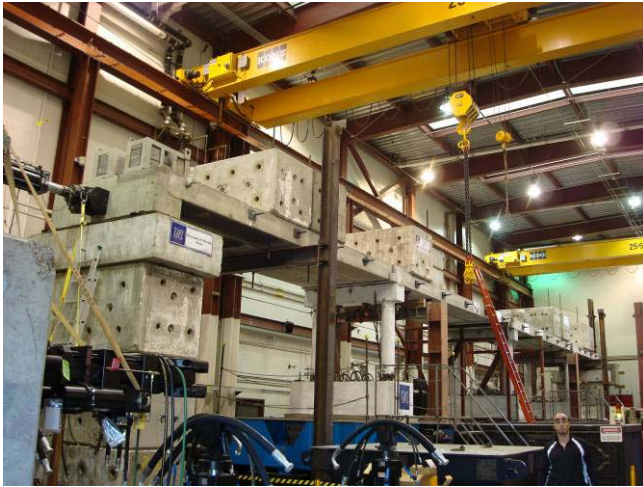
Figure 5. Testing a four-span, quarter scale, bridge on the NEES shake tables at the University of Nevada Reno.
