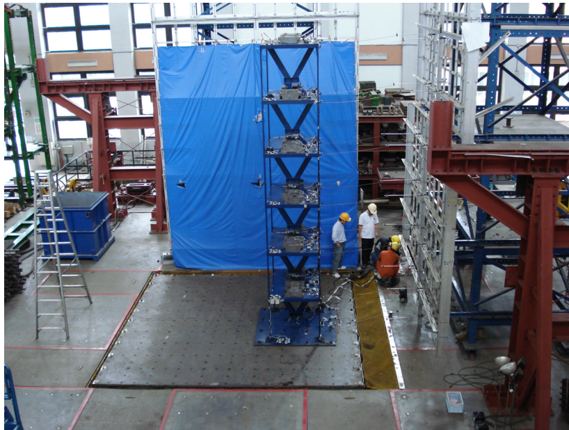
Figure 2. Six-story steel frame structure mounted on a six degree of freedom shake table at the National Center for Research on Earthquake Engineering (NCREE), Taipei, Taiwan. One MR damper is installed on each story using a V-brace. Wireless sensors are coupled with each MR damper to measure story accelerations, communicate measurements, calculate control forces and issue commands to the MR dampers.
