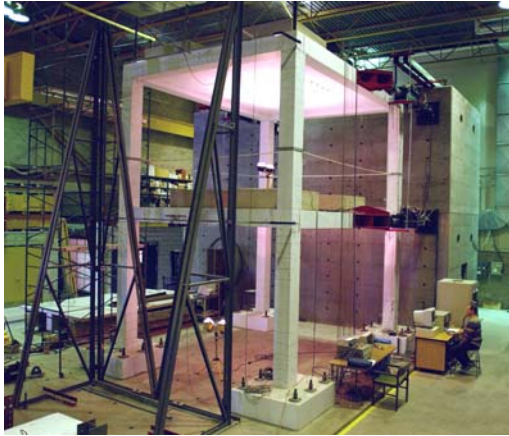
Fig. 8: Pseudo dynamic test on a full size two-story high-strength concrete frame.
