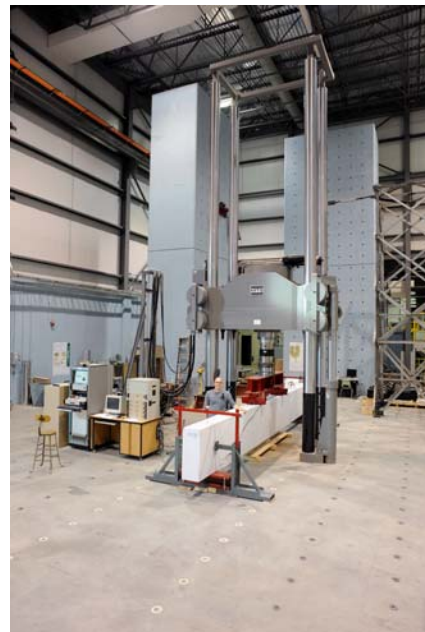
Fig. 7: Test on a large fiber-reinforced concrete beam, 12m high reaction walls are in the background
