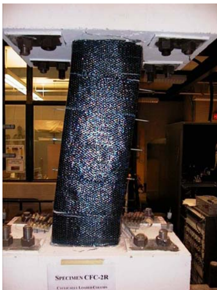
Figure 15. Testing of rehabilitated column at McMaster
