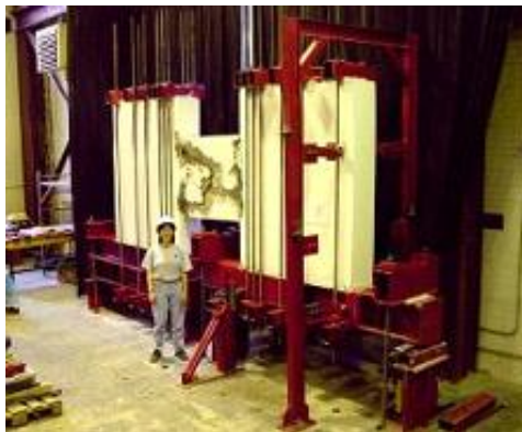
Figure 1. Frame for testing wall panels, McGill
