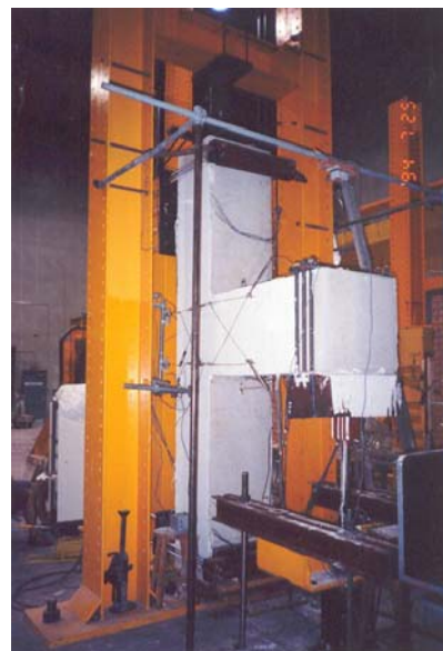
Figure 16. Testing of beam column joint at McMaster
