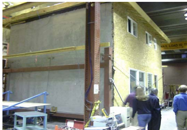
Figure 17. Shake table test on a full-scale two-storey house
