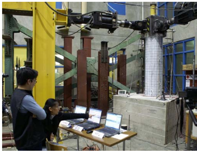
Figure 11. Hybrid multi-site test on bridge column
