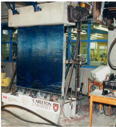
Figure 10. Test on concrete shear wall strengthened with carbon fiber
