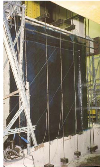
Figure 13. Surface bonded FRP on masonry infill
