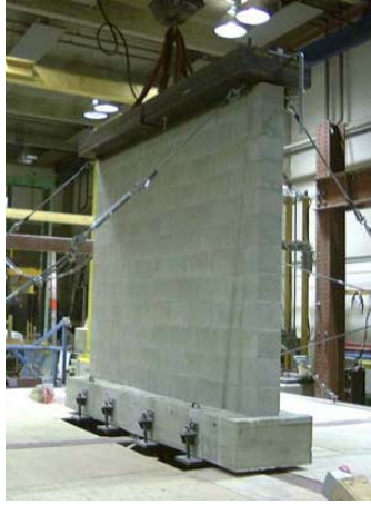
Figure 17. Retrofitted masonry wall on the shake table
