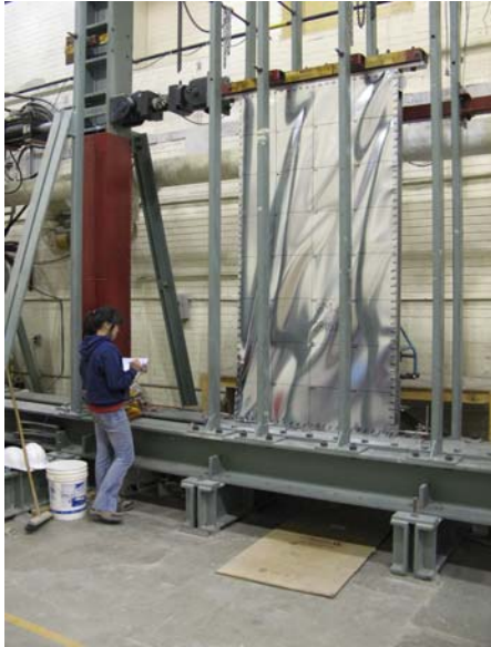
Figure 2. Steel sheathed old-formed steel framed shear wall test at McGill
