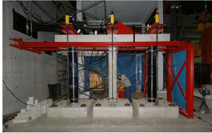
Fig. 9: Pseudo dynamic substructure test of 1/3 scale three-columns bridge pier.
