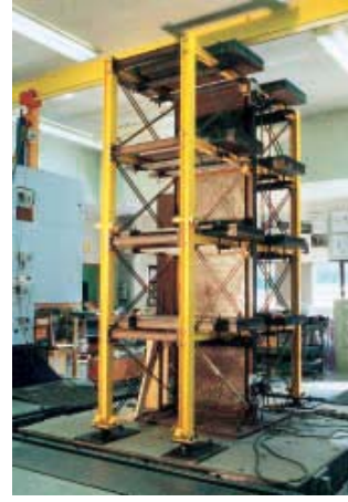
Figure 18. Shake table test on a wood panel wall
