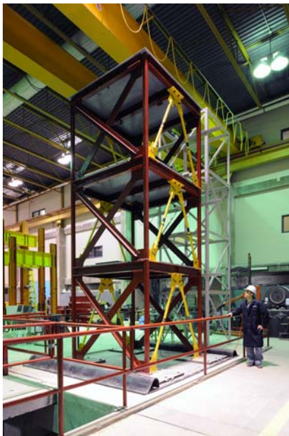
Fig. 6: Pseudo dynamic test at Sherbrooke on a 3-storey Steel frame with Chevron bracing
