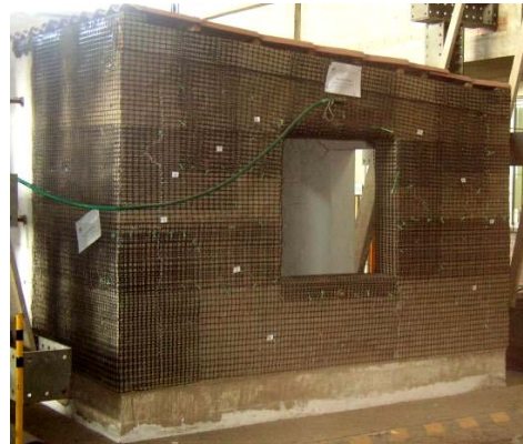
b) Reinforced adobe house after shaking test
