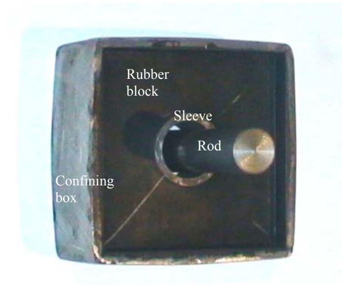
Figure 2. Bonded rubber unit (BRU) with inner steel rod.
