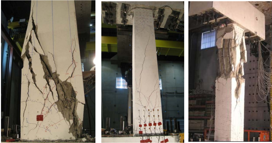
Figure 3. (a) Specimen 1 after axial failure (b) Specimen 2 after axial failure (c) Specimen 3 after axial failure
