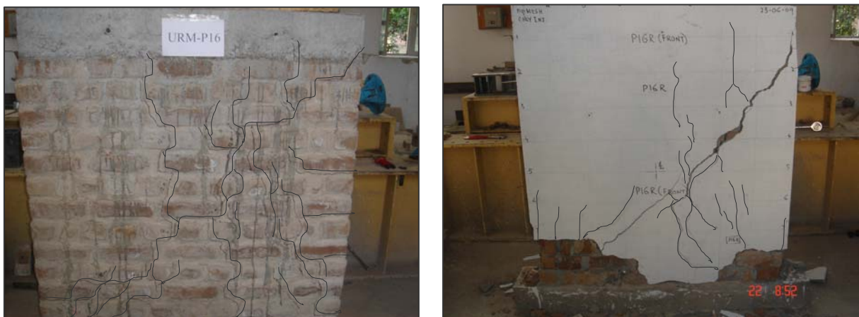
Figure 11. Final damage photograph of specimens P16 (left) and P16R (right)
