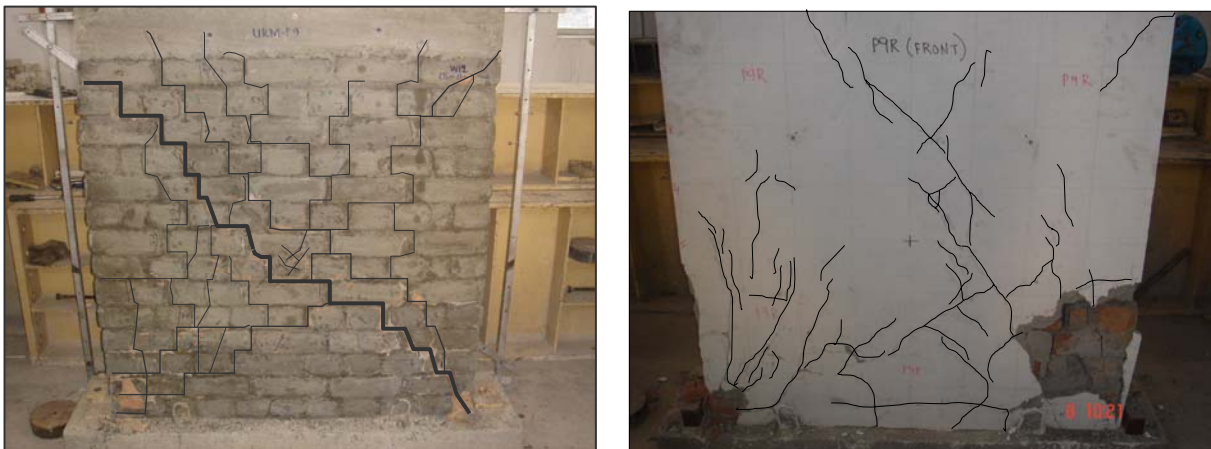
Figure 9. Final damage photograph of specimens P9 (left) and P9R (right)
