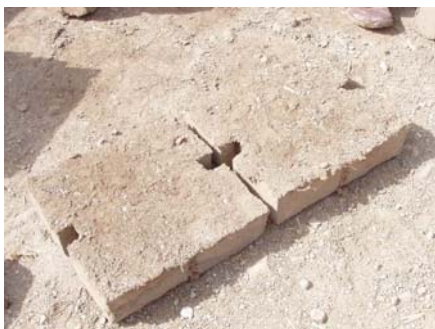
Figure 13 Adobe bricks manufactured in Huangascar. Space for vertical cane is larger than that of the original method
