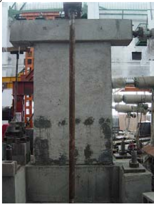
Figure 8. Test setup for RC shear wall specimen.
