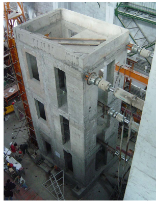
Figure 12. Test setup for three-story prefabricated RC shear wall structure.
