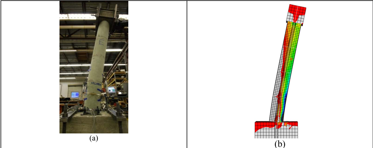
Figure 4: Deformed shape of FRP4 (a) from the experimental work, and (b) from the FE modeling
