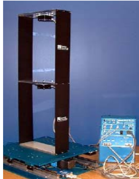
Figure 1. Shake Table Experiment
