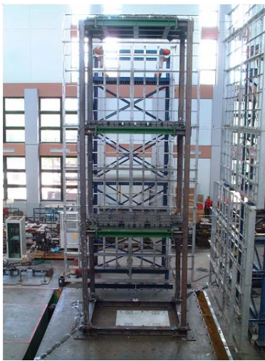
Figure 3. Photo of the three-story steel frame.
