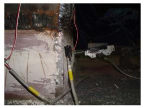
Figure 8. Local Buckling of West Column (West Side) at 2.2% Drift
