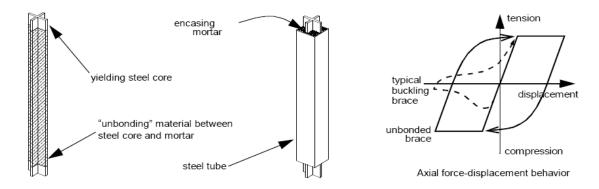
Figure 3. Schematic Mechanism of the BRB (Clark et al. 2000)
