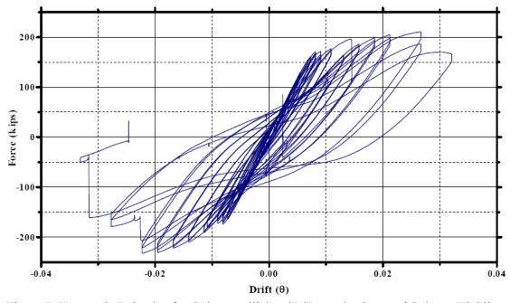
Figure 7. Hysteretic Behavior for Column utilizing SPSLs at the Onset of Column Yielding
