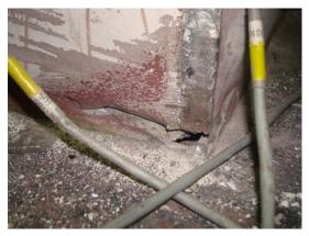
Figure 9. Fracture of West Column (North West Corner) at 2.7% Drift
