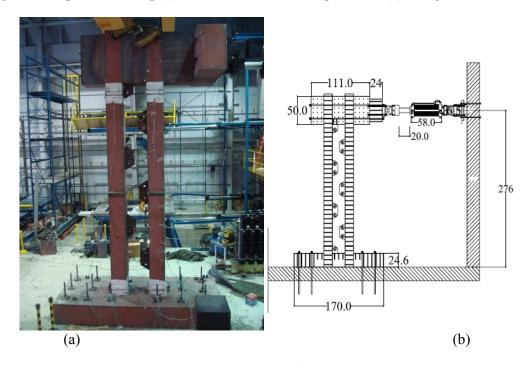
Figure 6. Experiment Setup (a) General View of the Experiment, (b) Bare Bridge Pier
