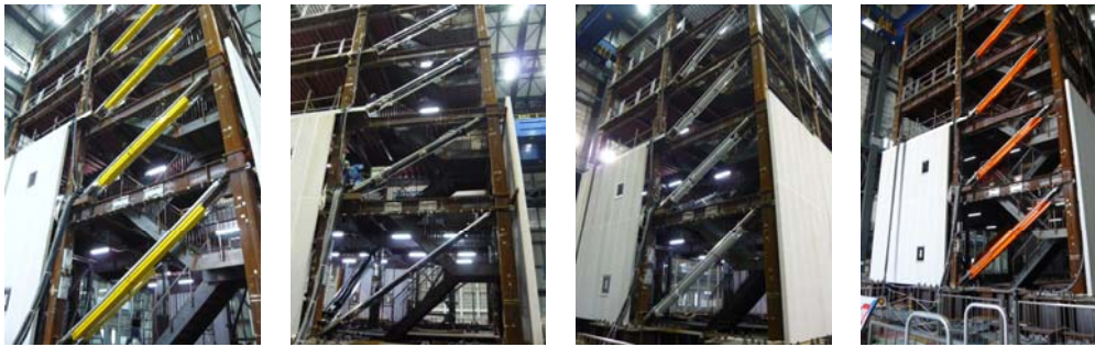
Figure 7. Four types of damper inserted in the building specimen (Steel, viscous, oil, and viscoelastic dampers, respectively)
