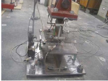
Fig 7. Tee stub experimental test
