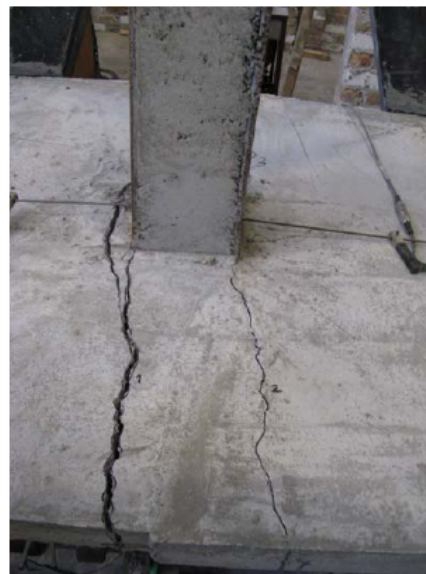
Fig 12 . The Location of weakest point of connection Fig 13. Crack Pattern across the slab
