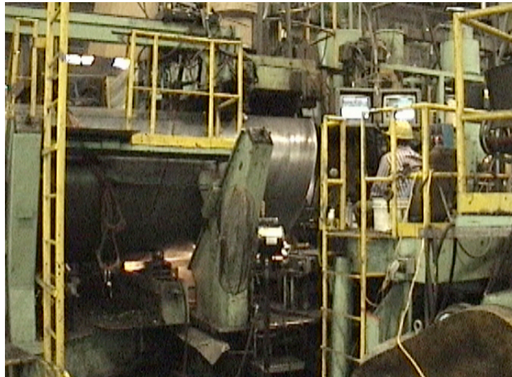
Figure 9. Spirally welded tube manufacturing process
