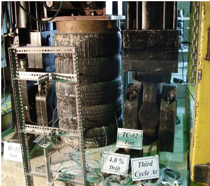
a) Column at 4% lateral drift
