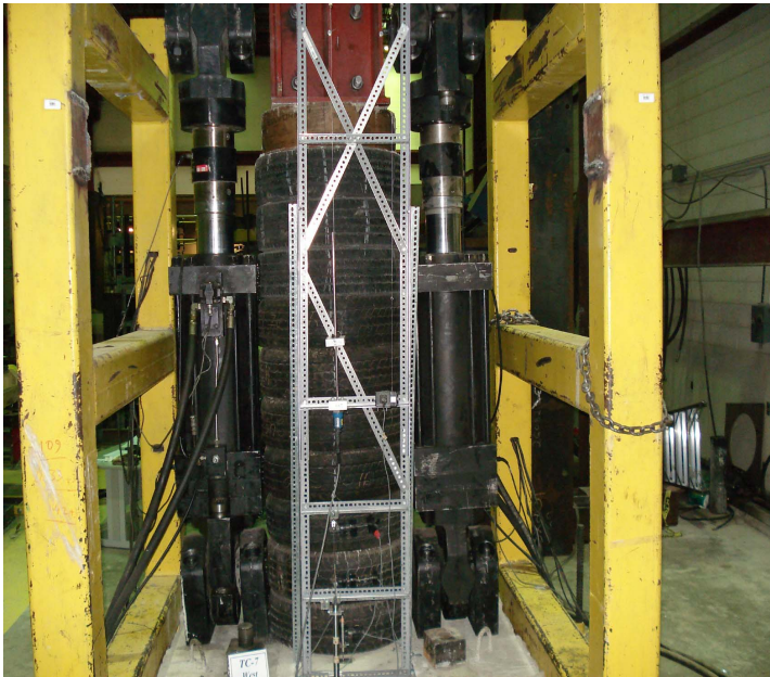
a) Column at 2% lateral drift
