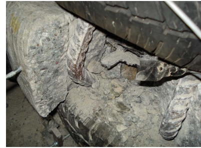
c) Bar buckling at the end of test
