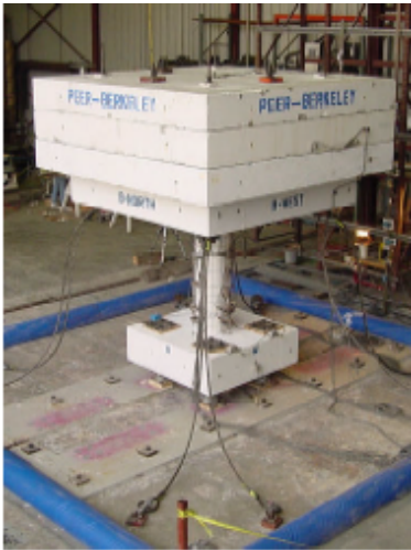
a) Picture of the prototype model on the EERC shaking table.
