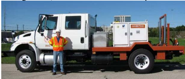
e. Urban, three-axis shaker called Thumper
