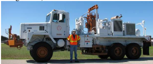
c. Single-axis, vertical shaker called Raptor
