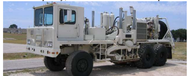
d. Single-axis, horizontal shaker called Rattler
