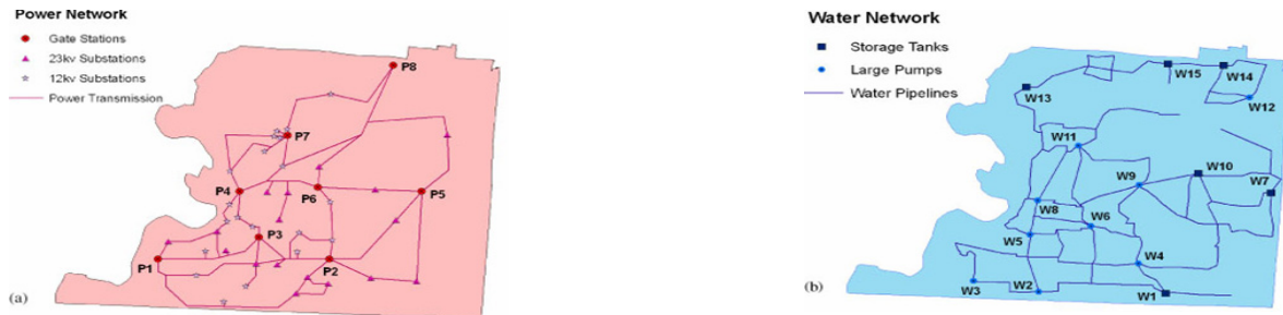
Figure 1. Topological structure of the lifeline networks in Shelby County, TN: (a) electric power grid; and (b) potable water distribution networks
