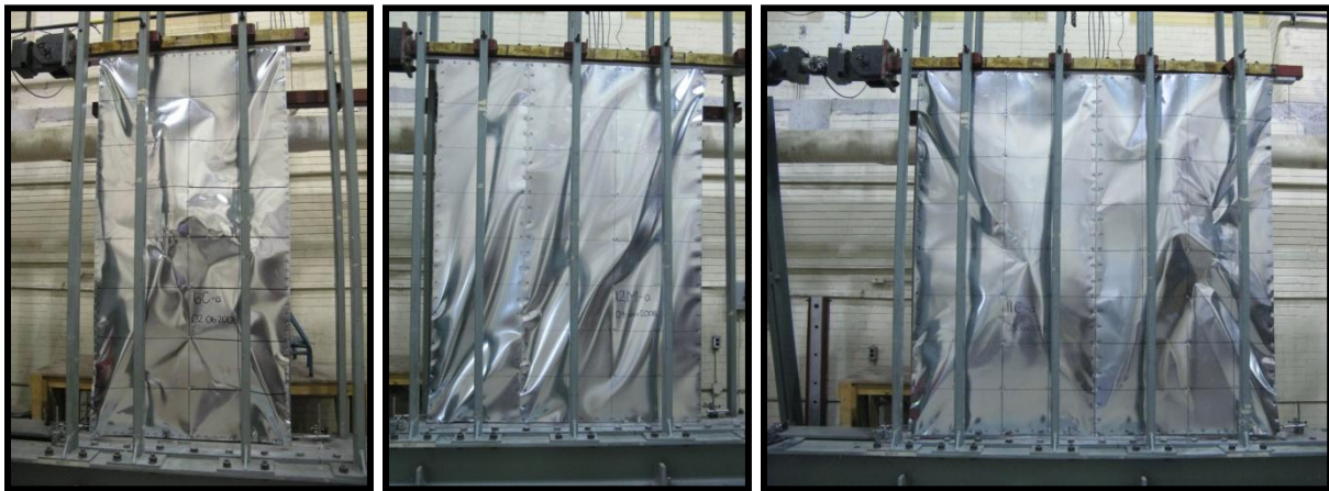
Figure 2. Shear wall test specimens showing tension field and elastic shear buckling deformations in steel sheathing.
