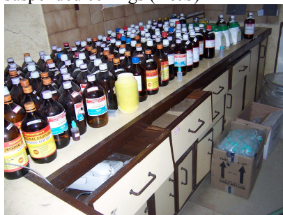
(g) Wrong storage of chemicals (H)
