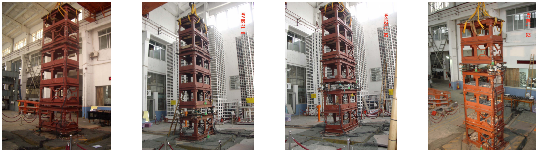
(a) base isolation (b) bottom of 2 nd st. (c) bottom of 3 rd st. (d) bottom of 5 th st.
