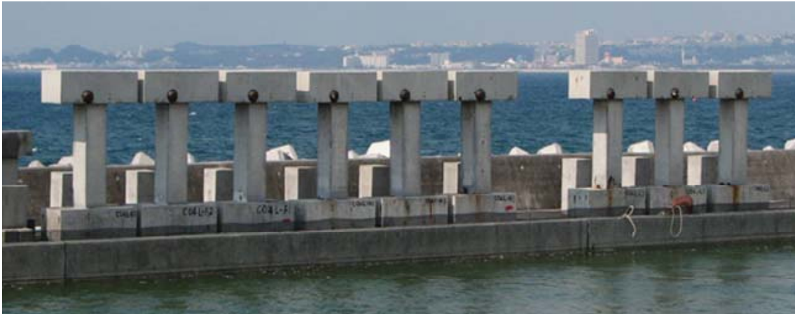
Figure 2. Exposure of RC column specimens in Okinawa seashore
