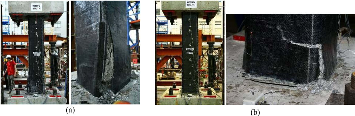
Figure 13. Failure modes of the specimens in Group 2 (a) R08RF3 (b) R08RF4
