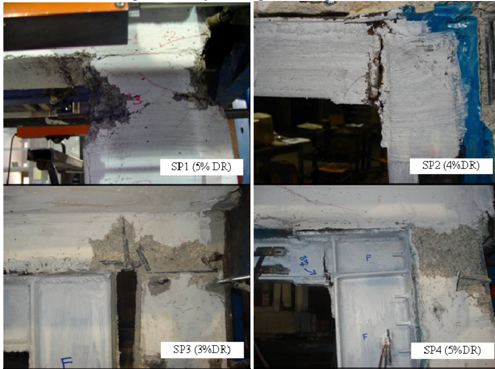
Figure 4. Cyclic response of specimens
